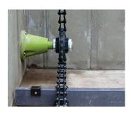
Wide profile static sleeve bearings are assembled with the use of clamping bands that pull the two halves togeather without the need for nuts and bolts. They are designed to work with 5.25" LTB sprockets such as MAXCO Chains's Cast Nylon Sprockets.
