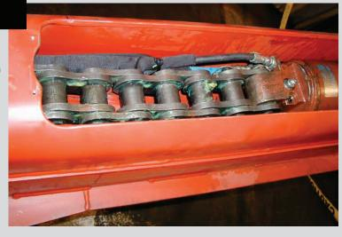
SEAL GUARD™ Roller Chains are available with a variety of corrosion resistant coatings. Our unique Inspire Series™ stainless steel blast coating is standard finish, optional black oxide or our Perfect Coat Plus II® surface treatments offer significant added protection against external chain corrosion.
