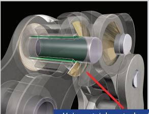
Construction, mining, shot blast equipment, as well as a broad range of heavy duty roller chain applications can now utilize large pitch roller chain - Sizes 60 (3/4"pitch) thru 240 (3" pitch) and enjoy the significant benefits of maintenance free operation. The unique stainless steel contact seals, installed between the link plates, retains a high quality bearing grease inside the chain joint, keeping out damaging abrasives such as grit and other debris that decrease chain life.
